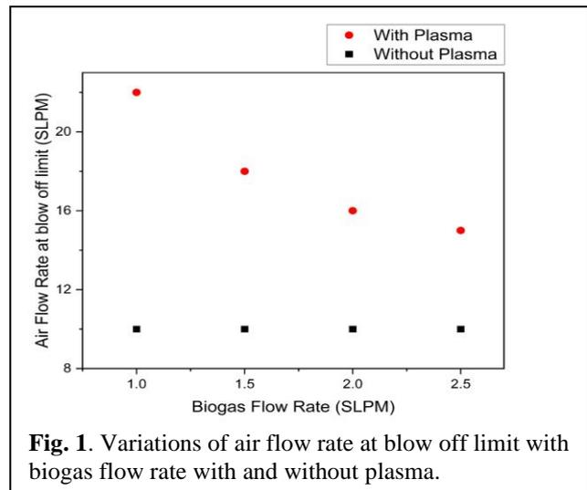
**Fig. 1.** Variations of air flow rate at blow off limit with biogas flow rate with and without plasma.
